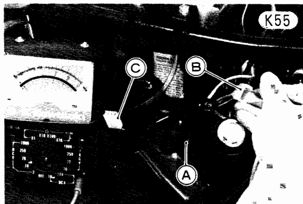
A. Brake Light Failure Indicator Switch B. 3-pin Socket C. 3-pin Plug
