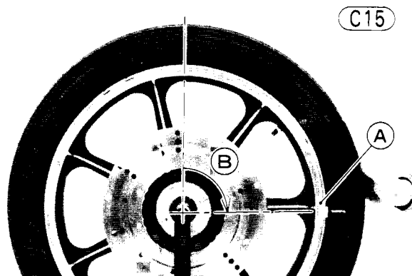
A. Balance Weight B. \frac{1}{4} Turn
